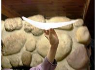
Even though you did not put dihedral into the wing when you taped it, the foam is thin. Once it is in flight the lift will bend the foam to have a little dihedral in the wing. You can also try a board launch.
