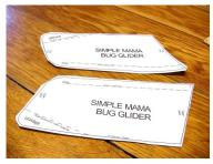
The wing pattern enclosed by the solid black lines will fit on the sheet of foam, but just barely, if you place it perfectly. Put that "cut close" corner exactly on the corner of the foam. The "leading edge" of the pattern should be very close to the edge of the foam. Once you are sure that the inside of the pattern is all on, tape the pattern to the foam on the two ends where it says, "tape here". I used red tape just so it shows up on camera.
