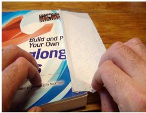
After folding the other side of the front camber the same way, put the pattern under the book cover with just the elevon (back flap) dashed lines barely peaking out (the paper pattern is on top and foam underneath again). This time, use a ruler or something similar and fold the elevons up and all the way over, 180 degrees again to establish
